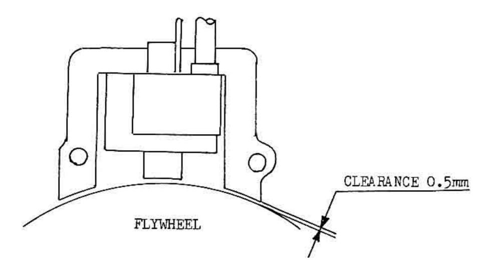
When installing the ignitor unit, the clearance to the flywheel should be set to 0.5 mm.
